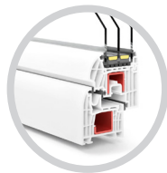
T-Classic Plus 8 chambers depth of frame: 70 mm
