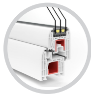
T-Classic 7 chambers depth of frame: 70 mm
